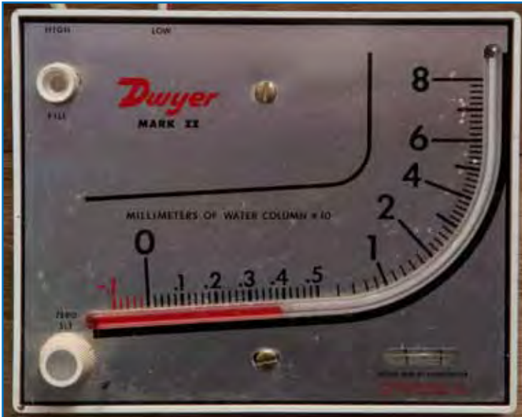
Figure 104: A manometer used to monitor air pressure within the house (the reading given is equivalent to 0.15 inches of water column).
