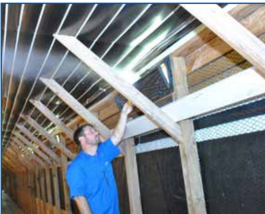
Figure 6.7: Using a smoke test to determine if airflow and operating pressure are correct.
