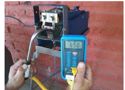
Pyrometer indicating proper blade temperature of 650°C.
